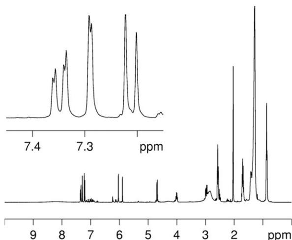
**Figure 4.**  $^1\text{H-NMR}$  spectrum of catechin dilaurate (**11a**) with expanded portion showing the B-ring signals.
