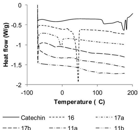
**Figure 8.** DSC thermogram (second heating cycle) of catechin laurates prepared by direct acylation (**16**, **17a**, and **17b**) and transesterification (**11a** and **11b**) compared with catechin.
