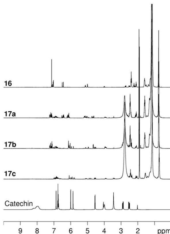
**Figure 5.**  $^1\text{H-NMR}$  spectra of catechin penta-, tetra-, tri-, and di-laurate (**16**, **17a**, **17b**, and **17c**) compared to unmodified catechin.
