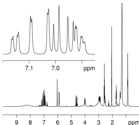
**Figure 3.** <sup>1</sup>H-NMR spectrum of 11b, with expanded portion showing the B-ring signals for catechin-3'-monolaurate and catechin-4'-monolaurate.
